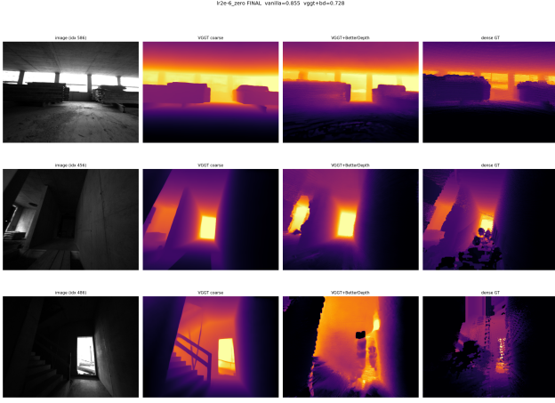
Figure 6: Depth maps comparison. The original VGGT depth maps (2 nd col.) have more fidelity to the scene (1 st col.) than our synthesized ground truth (4 th column). The BetterDepth refined results (3 rd col.) show the artifacts generated by our Ground Truth proxy.
